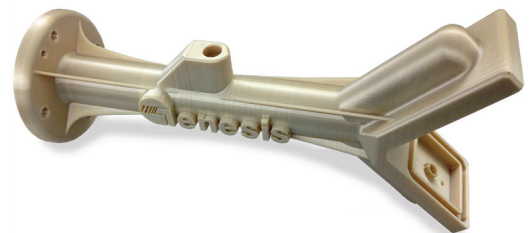
Figure 3: Custom EOAT with internal vacuum channels made with FDM material (ULTEM™ 9085 resin tan).
