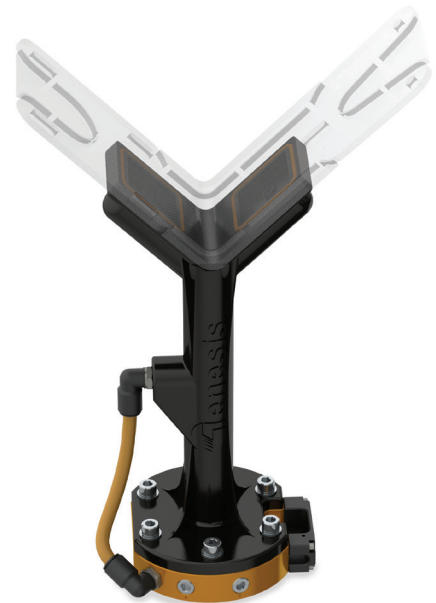
Figure 5: Example of EOAT (black) that leverages FDM's design freedoms.
