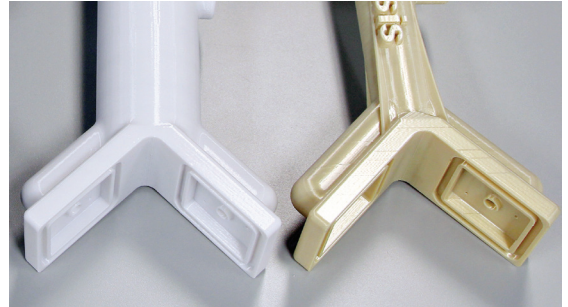
Figure 22: Genesis FDM EOAT iterations (left to right: PC White, and ULTEM™ 9085 resin tan).
