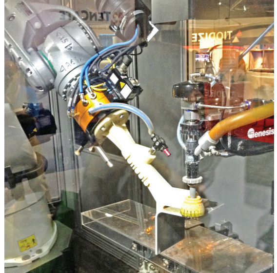
Figure 24: Single-piece, vacuum EOAT for waterjet cutting made with FDM material (ULTEM™ 9085 resin tan).
